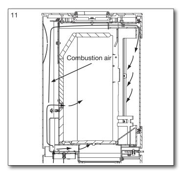
There is a risk of smoke escaping into the room if the door is opened during vigorous firing, or if there is a lack of air supply to the room, for ex. if an extraction fan is in use.
