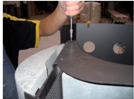
24. Remove the rear screw in the top plate.
