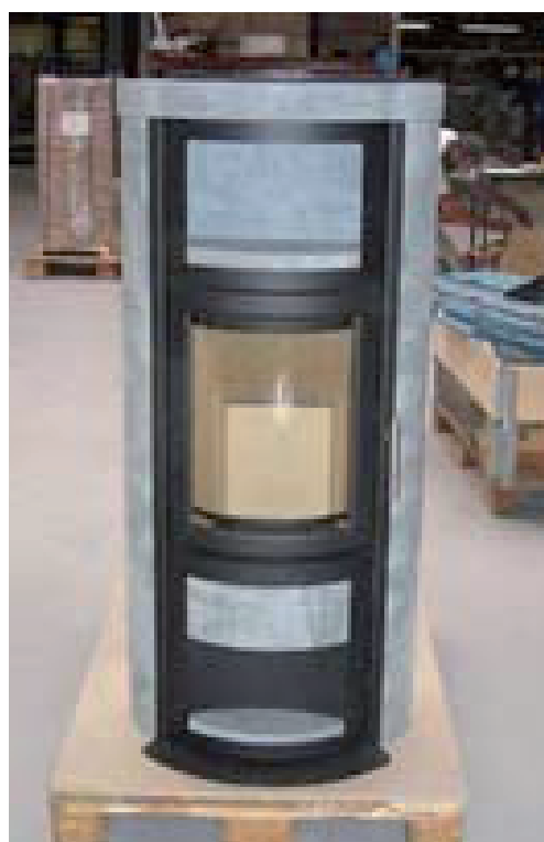
40. Installation of the Turin soapstone elements is complete.
