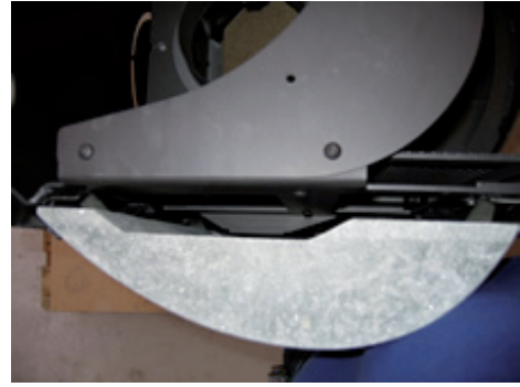
14. Correct position of the spring for the top stone.
