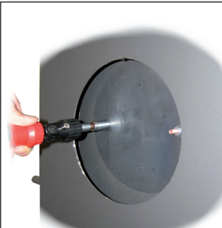
Fig. 2 Remove the two screws that hold the cover in place on the stove.
