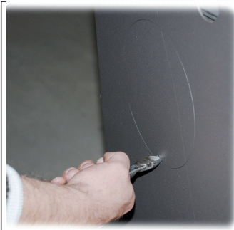
Fig. 1 Cut the small metal bridge connecting the cover to the back panel using side cutters. Then twist off the cover.
