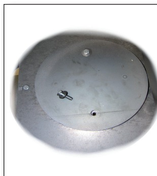
Fig. 10 Affix the cover using the appropriate bolts.
