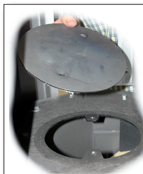
Fig. 9 Place the cover from the back outlet on top of the stove.
