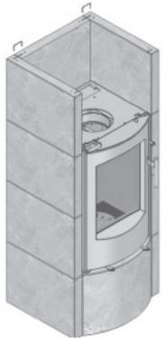
To continue, fit the next rear stone and both side stones. Position the brackets and pins into the holes.
