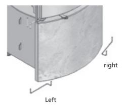
Fit both side stones, positioning the rear brackets under the soapstones. When fitting the right and left brackets onto the front and side soapstones, tip the stove backwards.
