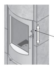
Regulate the convection air flow by turning the handle on the side of the stove.
