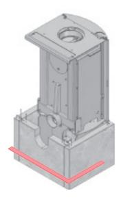
Then fit the rear stones and check that the soapstones are at right angles. Fit the next rear stone and both side stones. Position the brackets and pins in the holes in the soapstones
