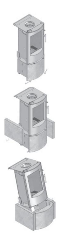
When the stove is positioned precisely, position the lower front stone up against the stove base leg and secure with 1 x right and 1 x left bracket.
